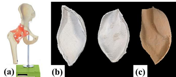
Fig. 8. (a) Anatomical functional model of the hip joint. (b) Example of a plaster mold. (c) Manufactured silicone muscle.
