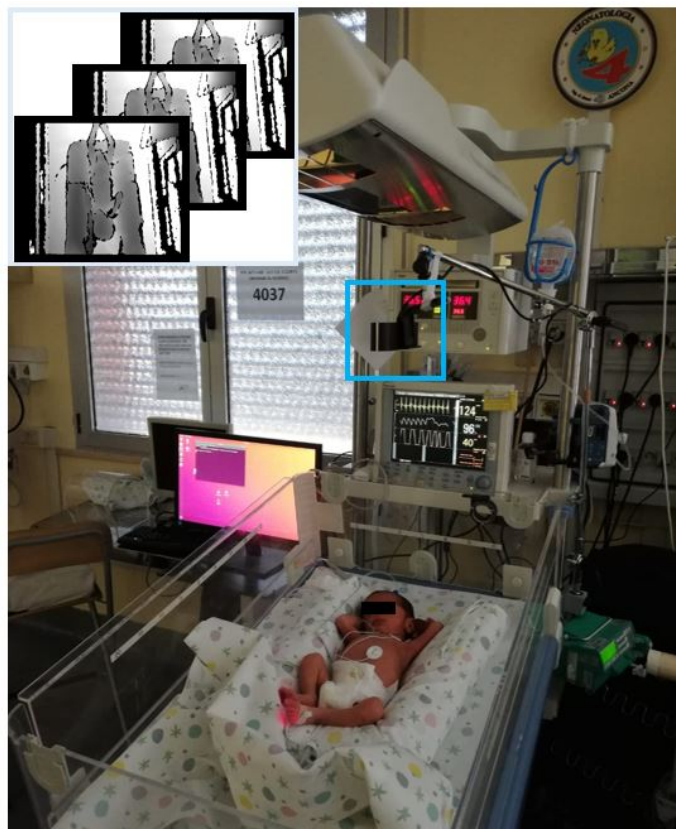
Fig. 1: Acquisition set-up: the RGB-D camera (light-blue box) does not hinder the healthcare team of the Neonatal Intensive Care Unit (NICU) during the actual clinical practice. An example of acquired depth stream is showed on top left.
