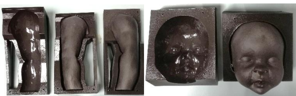
Fig. 2: Some moulds parts printed in PA-12 material.
