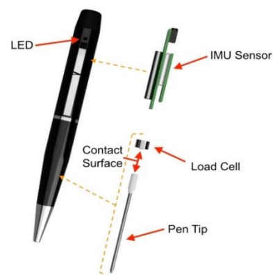
Figure 1. A rendered image of the ink pen and its internal components.
