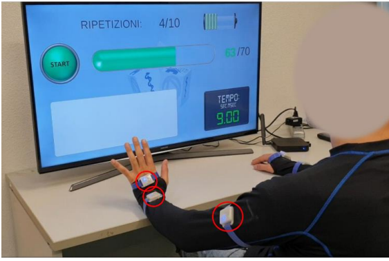
Figure 3. Example of serious interface. MIMUs are encircled in red.
