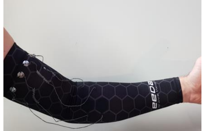
Figure 1. Sensorized polyester stretchable arm sleeve for sEMG applications.
