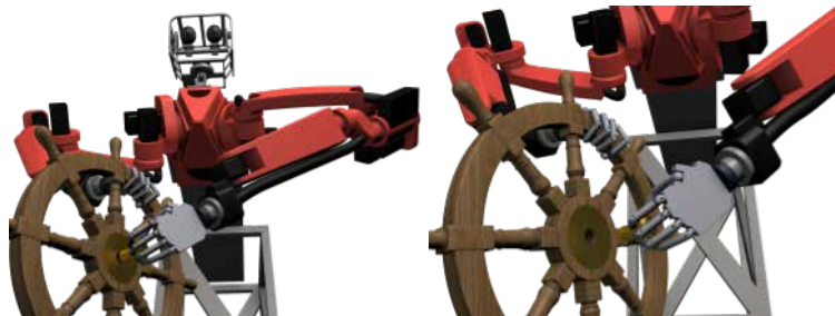
Fig. 3. A potential task in the Circular Economy: the dismantling of a ship's wheel. An exemplary task in the Circular Economy: the dismantling of a ship's wheel. The execution of this task without fixtures requires bimanual manipulation: the left hand holds the wheel, the right hand performs the disassembly tasks. Dismantling procedures require to cope with the disassembly of a large variety of mechatronic systems. Reducing the number of needed dedicated set-ups is key for the economic viability of the process.
