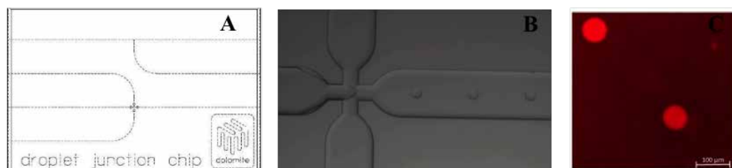
Fig. 1. Generation of PEG Droplet in the Microfluidic device. A. Microfluidic chip used in this work. B PEGDA microparticles (20%PEGDA). C. Fluorescent image of Fluorescein encapsulation.
